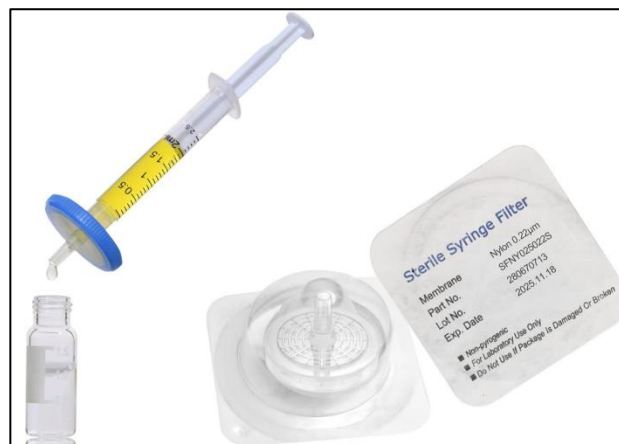
Figure 76. Sterilization by filtration using sterile syringe filters.
